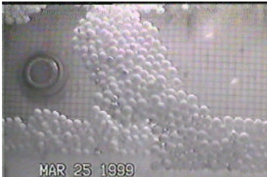
Figure 3. Aluminum Oxide spheres forming walls in '99 microgravity flight test. Note the fluctuating g-level causing the wall to shift.
