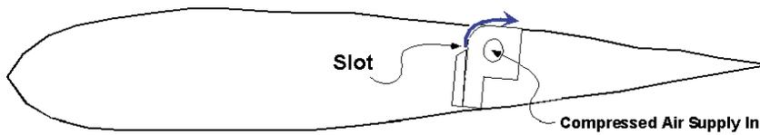
Figure 3b: Schematic of Airknife inside wing body
