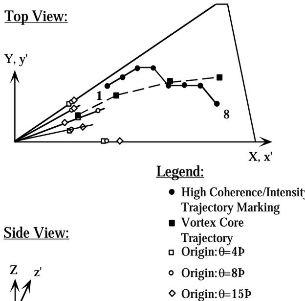
**Figure 7.** Trajectory of high coherence and energy for a 59.3 delta wing (Ref. 19).
