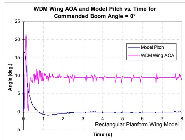
Figure 6: WDM control wing angle of attack and boom angle vs. time for commanded boom angle = 0° (rectangular planform wing model)
