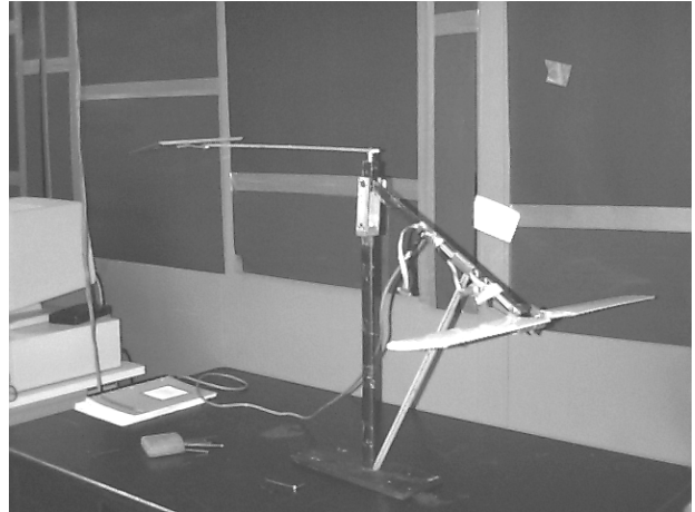
Figure 2: Pitch Manipulator used in the present experiments (with delta wing model attached)
