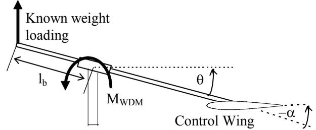
Figure 4: WDM-Generated moment direct calibration setup
