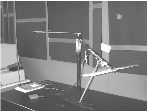
Figure 12: Pitch Manipulator used for delta wing lift measurements. From Ref. 19.
