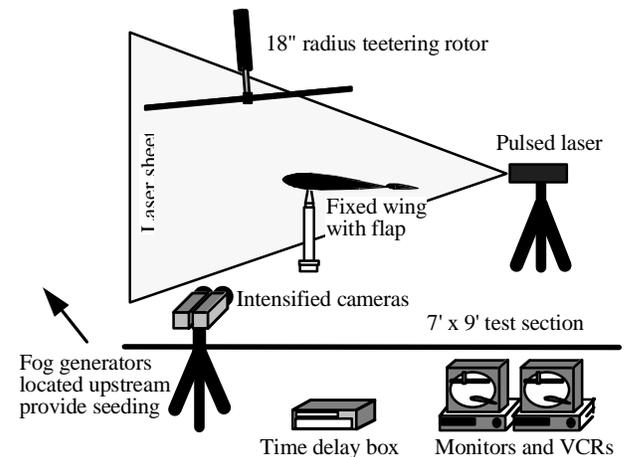
Fig. 1: Experimental set-up for wing-rotor
