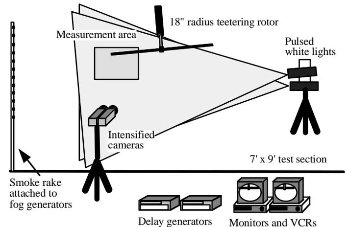
Figure 7: Experimental set-up for isolated rotor test in Harper Tunnel
