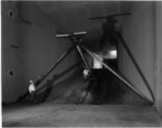
Figure 1: Rotor mounted in settling chamber of 7' X 10' wind tunnel
