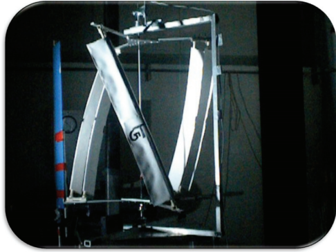
Figure 7: Blade deflection is visible in this strobe-lit snapshot of the 3-armed VAWT in operation. The blue guidevane is visible to the left.
