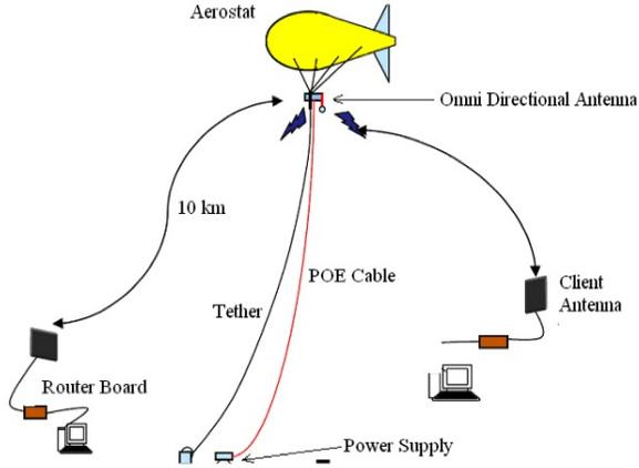
Fig. 1. Aerostat based wireless communications system. From [21]
