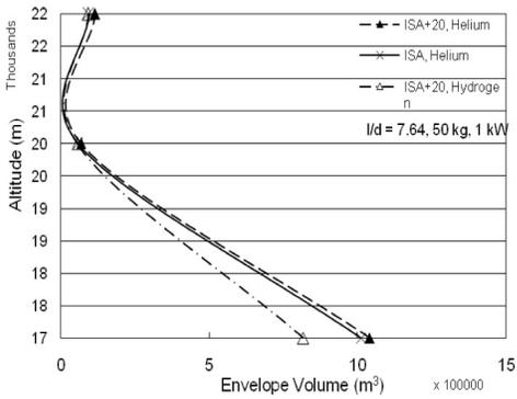
Fig. 3. Sensitivity of envelope volume to operating altitude
