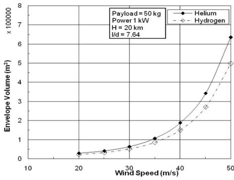
Fig. 2. Sensitivity of envelope volume to ambient wind speeds
