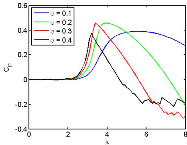
Figure 9. Power coefficient vs. tip speed ratio for various solidities of the 6 ft VAWT ( $U_\infty = 12$  m/s,  $\lambda = 1$ ).
