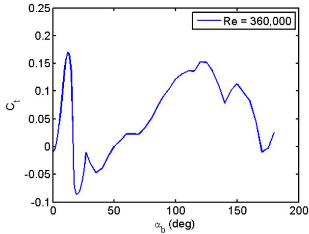
Figure 11. Tangential coefficient vs. blade angle of attack for a NACA 0015 airfoil.
