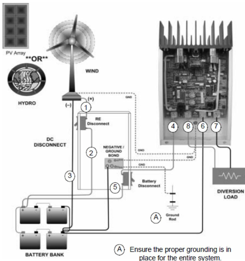
Figure 5. Diversion control mode wiring.
