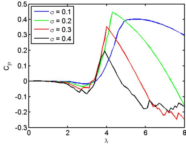
Figure 8. Power coefficient vs. tip speed ratio for various solidities of the 3 ft VAWT ( $U_\infty = 12$  m/s,  $\lambda = 1$ ).
