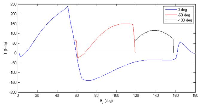
Figure 13. Torque vs. blade azimuth angle for various guide vane angles of attack of the 6 ft VAWT ( $U_\infty = 12$  m/s,  $\lambda = 2$ ).
