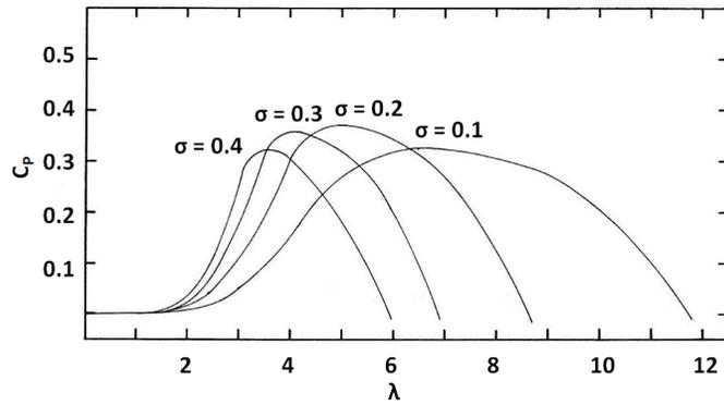
Figure 2. Power coefficient vs. tip speed ratio for various solidities (Sandia).<sup>4</sup>
