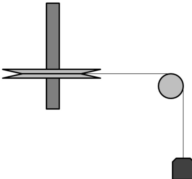
Figure 7. Rope brake dynamometer.
