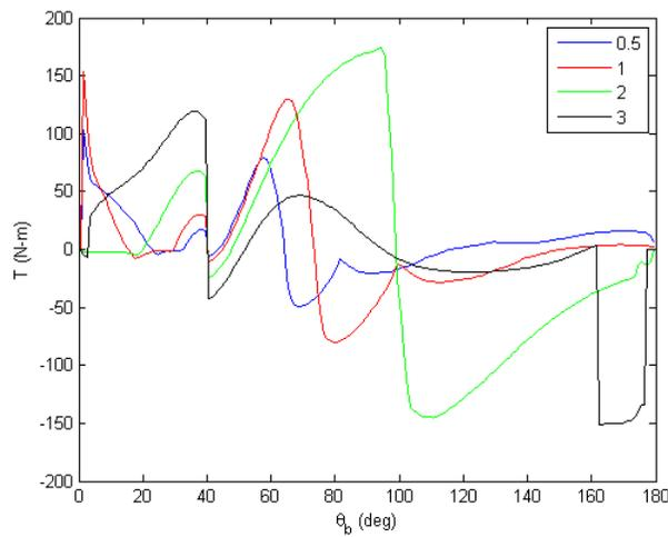
Figure 12. Torque vs. blade azimuth angle for various tip speed ratios ( $U_\infty = 12$  m/s,  $\alpha_g = -40^\circ$ ).
