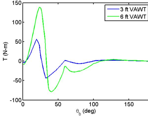
Figure 10. Simulated variation of torque with blade azimuth angle ( $U_\infty = 12$  m/s,  $\lambda = 1$ ).
