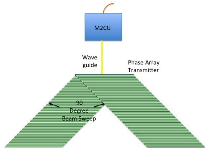
**FIGURE 4.** The phase array transmitter will be able to sweep the beam 45 degrees fore and aft, and 10 degrees side to side.
