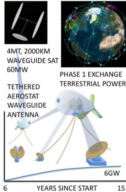
**FIGURE 1.** In Phase 1, a 2000 km constellation of 100 waveguide satellites of 4000kg each is built over 9 years, transacting 60MW power each, between terrestrial power plants and customers. Waveguides inside aerostat tethers minimize atmospheric losses.
