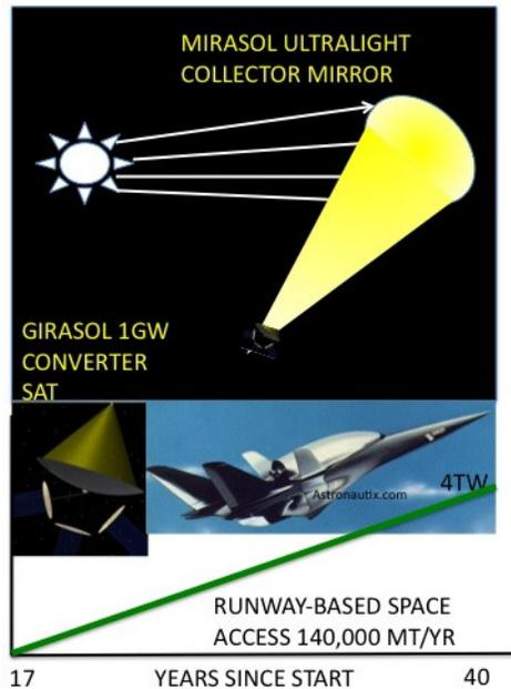
**FIGURE 2.** In Phase 2, a 2GW ultralight Mirasol sunlight collector and a 1GW, 220GHz Girasol Brayton cycle converter, in orbits near 2000 km, form the standard component of a Space Solar Power constellation, growing to over 4 TeraWatts of SSP by Year 40. The Earth link system is expanded from Phase 1 with minimal technical risk.
