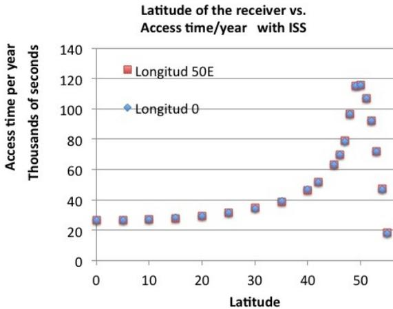
**FIGURE 9.** Variation of power beaming link time per year with latitude
