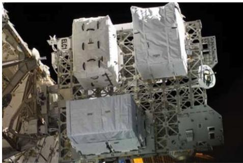
**FIGURE 7.** Typical mounting of ELCs at the ISS. From the NASA ISS Reference Manual, courtesy NASA
